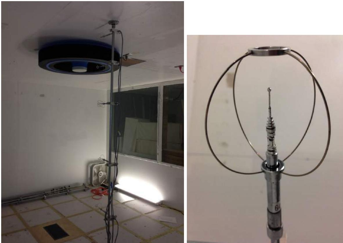
Figure 1. Exhale bladeless fan installed in the test space and air velocity sensor.
